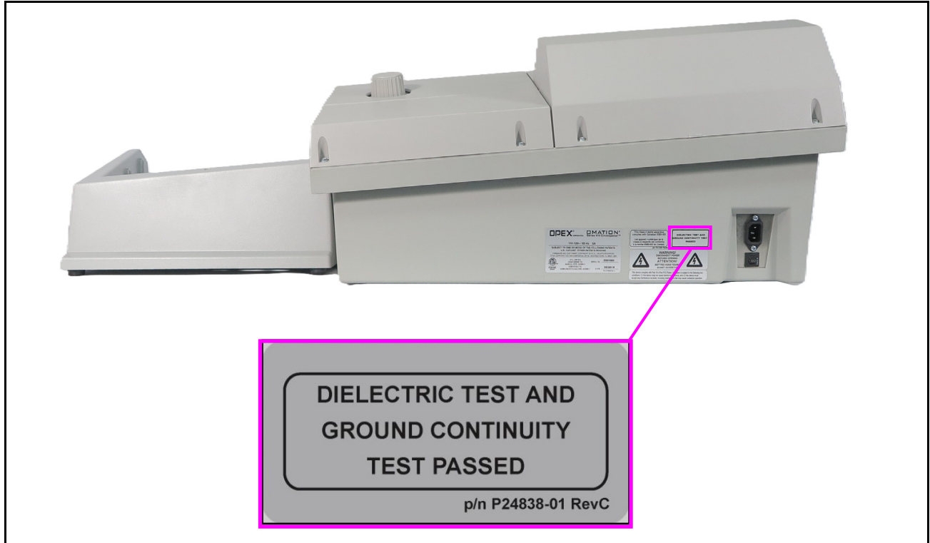
Figure 1-6: Dielectric and Ground Test Label P24838-01
