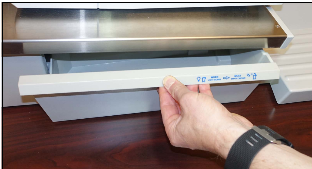
Figure 1-2: Bin tray removal interlock triggering
