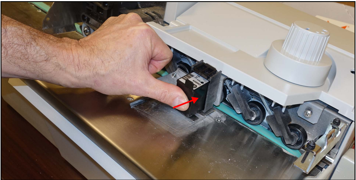
Figure 4-6: Replacing the printer cartridge
