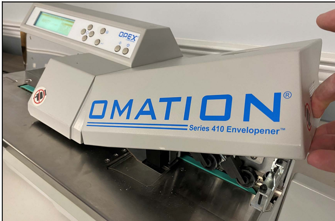
Figure 4-2: Lifting the Nip arm cover
