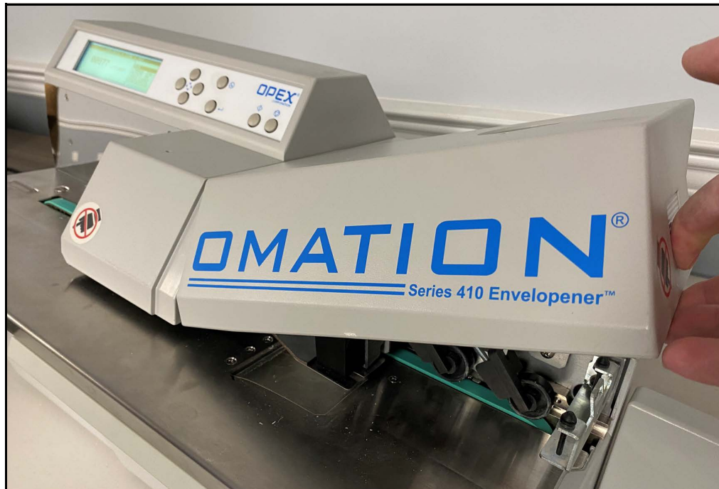
Figure 1-1: Top cover removal interlock triggering
